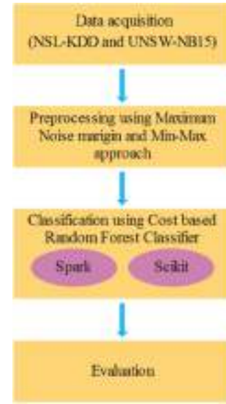
Fig. 1. Block diagram of CRFC-IDS method.
